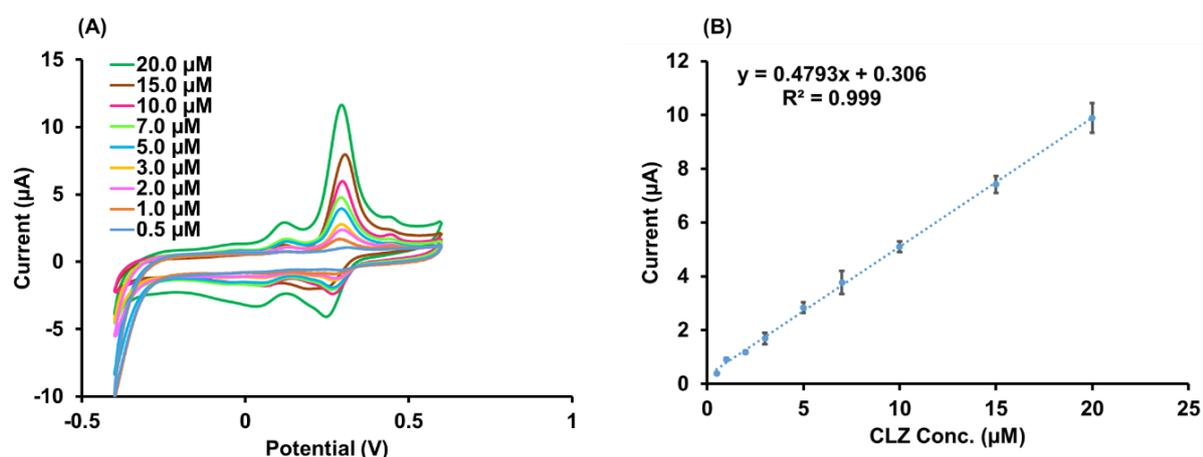
Fig. 4 (A) The CV current responses of RuO<sub>2</sub>/Au/MWCNT/SPE modified electrode for various concentrations of CLZ from 0.5 to 20 μM (0.5, 1.0, 2.0, 3.0, 5.0, 7.0, 10.0, 15.0 and 20.0 μM) in 0.1 M BRS buffer solution, pH 7.0 at scan rates 50 mV/s<sup>-1</sup> respectively. (B) The calibration plot presents the relationship between the CV peak current (μA) and the concentrations of CLZ (μM).
