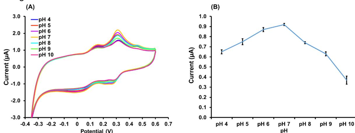
Fig. 3 (A) CV responses of  $\text{RuO}_2/\text{Au}/\text{MWCNT}/\text{SPE}$  modified electrode in BRS buffer solution at different pH value between 4 to 10. (B) Plot of current ( $\mu\text{A}$ ) versus different pH values between 4 to 10.
