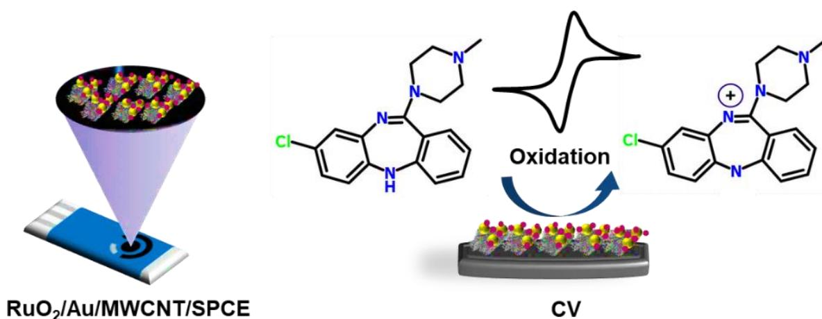
Fig. 1 The schematic of SPE modification with RuO<sub>2</sub>/Au/MWCNT nanocomposite for CLZ determination.
