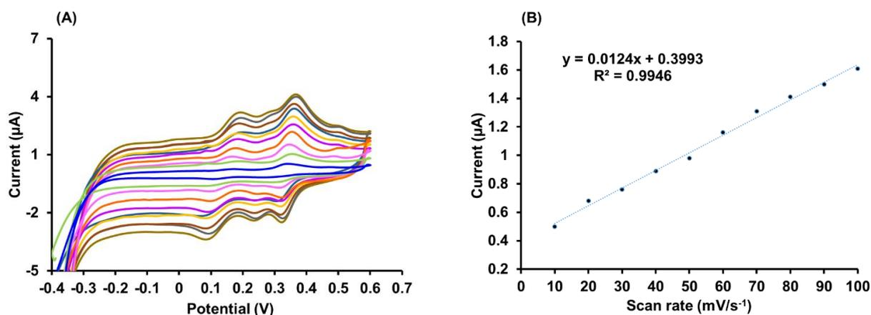
Fig. 2 (A) The CV current response of RuO<sub>2</sub>/Au/MWCNT/SPE in BSR buffer solution at pH 7 containing 1.0 μM CLZ at various scan rates between 10 to 100 mV/s<sup>-1</sup>, respectively. (B) The plot of variation of CV peak current versus different scan rates.
